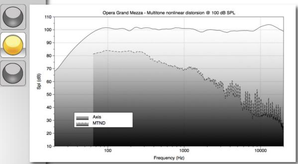
As can be seen in the graphic which represents the instantaneous harmonic distortion, mapped by monitoring acoustic pressure and the displacement of the membrane at the same time, a sweep of 8 V generates a positive offset of about 2.5 mm, and highlights the rather abrupt limiting of the suspension of the woofers for nega-
