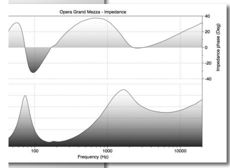
The impedance module shows parallel at low frequencies of the two woofers, with a minimum a little over 3 ohms just above 150 Hz; at these frequencies the phase is the negative zone, so here we find the maximum load conditions for the amplifier, in a fraction of the spectrum rather rich in energy content. Even here, therefore, it's necessary to pay attention to the interfacing with the amp, which must be stable at low impedances. A
